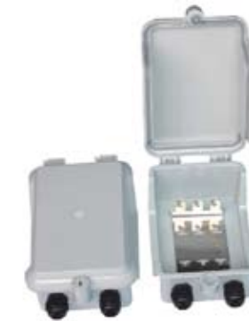
TRJK95 30 pair outdoor distribution box The box with 3pcs 10 pair LSA modules for outdoor condition,with key lock Plastic Parts: ABS. Mount frame:1mm thickness stainless steel. Size: 215mm × 85mm × 135mm.
