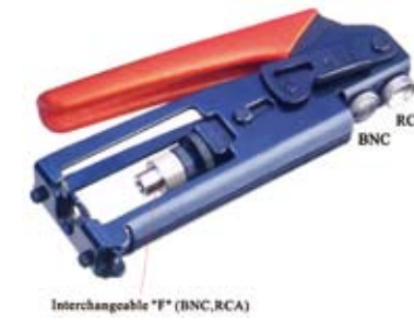
PBTL-5086(5.6"/142mm) For Waterproof Connectors Crimping Tool F/BNC/RCA RG-58/59/62/6(3C/4C/5C) Compressed Distance: F connector:15.8- 25 .8mm BNC connector:28.2- 38.2mm RCA connector:28.2- 38.2mm
