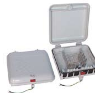
TRJK98 50 Pair Pouyet Type Distribution Box Dustproof, waterproof, ultraviolet radiation resistant Capacity of box 5pcs 10 pair LSA modules Housing material: ABS or Polyethylene Mount frame:1mm thickness stainless steel. Size: 264mm × 240mm × 76mm.
