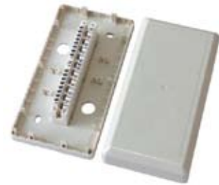
TRJK104 10 pair Connection Box With 10 pair disconnection module Material: ABS. Size: 160mm × 85mm × 36mm.
