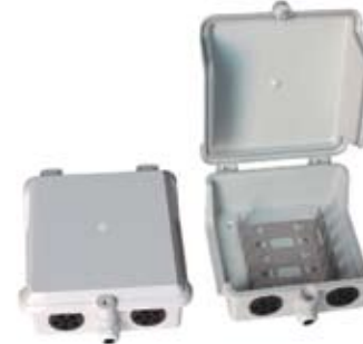
TRJK94 50 pair outdoor distribution box The box with 5 pcs 10 pair LSA modules for outdoor condition,with key lock Plastic Parts: ABS. Mount frame:1mm thickness stainless steel. Size: 220mm × 95mm × 190mm.
