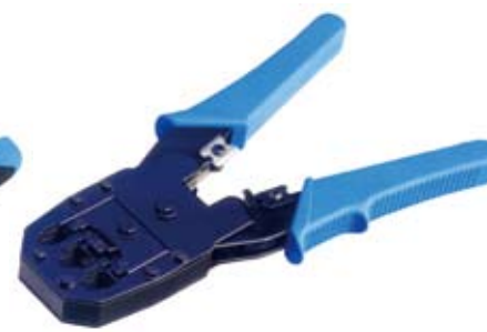
PBTL-315(7.7"/195mm) For crimping modular plug 8P8C/RJ-45,6P6C/RJ-12,6P4C/RJ-11 & 6P2C,4P4C & 4P2C
