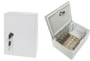
TRJK106 50 pair indoor distribution box Capacity of box 5pcs 10 pair LSA modules with 4 pcs wire ring and key lock Housing material: ABS. Mount frame:1mm thickness stainless steel. Size:210mm×160mm×90 mm.
