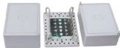
TRJK107 50 pair indoor distribution box for BT Capacity of box 5pcs 10 pair LSA disconnection modules Housing material: ABS plastic. Mount frame:1mm thickness stainless steel. Size: 208mm × 157mm × 90 mm.
