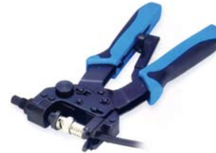
PBTL-H510B(7.7"/195mm) For F, BNC, RCA, right angled and keystone module compression connectors, Available for RG59 and RG6 cables. With adjustment for crimping different length of connectors.
