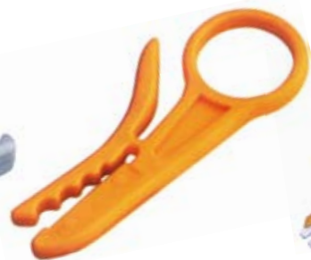
PBTL-308M (3.2"/82mm) Easy Stripper for UTP/STP Telecom Wire For stripping wire diameter \phi 5-\phi 6.2\text{mm} . Made of poly resin, economic type
