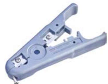
PBTL-S501A(4.8"/122mm) Multi-function cable stripper For UTP/STP wire and multi conductor cable from 3.2mm-9mm max.Irregular out-shape insulation can be put into the front "V"and "U" guide, rotate the tool 1-3 times by index finger for stripping the outer insulations easily.
