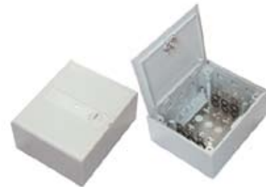
TRJK2049 30 pair indoor distribution box Mounted with 3pcs 10 pair LSA modules. with wire ring and coin lock Plastic Parts: ABS. Mount frame:1mm thickness stainless steel. Size: 170mm × 140mm × 75mm.
