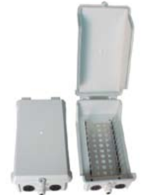
TRJK96 100 pair outdoor distribution box The box with 10 pcs 10 pair LSA modules for outdoor condition,with key lock Plastic Parts: ABS. Mount frame:1mm thickness stainless steel. Size: 400mm × 120mm × 195mm.
