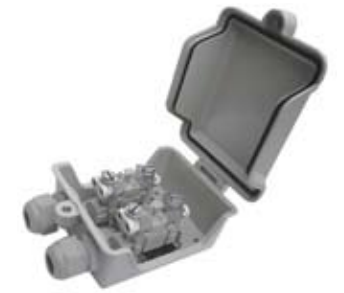
TRJK92 2 Pair Distribution Box With 2 pcs STB modules and screw lock Plastic Parts: ABS. Size: 139mm × 96mm × 55mm.
