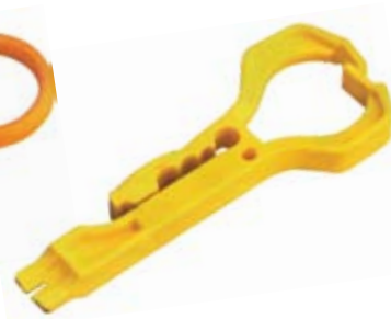
PBTL-328M (3.5"/89mm) Easy Stripper for UTP/STP Telecom Wire For stripping wire diameter \phi 5-\phi 6.2\text{mm} . top end for 110/88 type insertion use.
