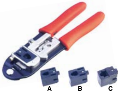
PBTL-3686(7.9"/200mm) For crimping modular plug A:4P4C & 4P2C B:6P6C/RJ-12,6P4C/RJ-11 & 6P2C C:8P8C/RJ-45
