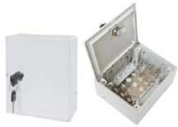
TRJK102 30 pair indoor distribution box Capacity of box 3pcs 10 pair LSA modules with 4 pcs wire ring and key lock Housing material: ABS. Mount frame:1mm thickness stainless steel. Size: 170mm×140mm×75 mm.
