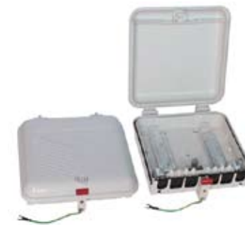
TRJK99 10 Pair Distribution Box 3M Pouyet type Dustproof, waterproof, ultraviolet radiation resistant For STB module,with screw lock Plastic Parts: ABS or PC Size: 264mm × 240mm × 76mm.
