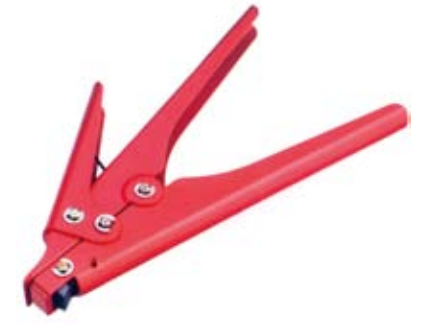
PBTL-519(7.5"/191mm) Cable Tie Fasten Tool For cable tie thickness up to 2.3mm & width up to 9.5mm with single spring loaded and comfortable hand force
