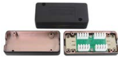
TRJK4105H Half-shielded spray-paint inside box Krone IDC block Size:84x37x23mm
